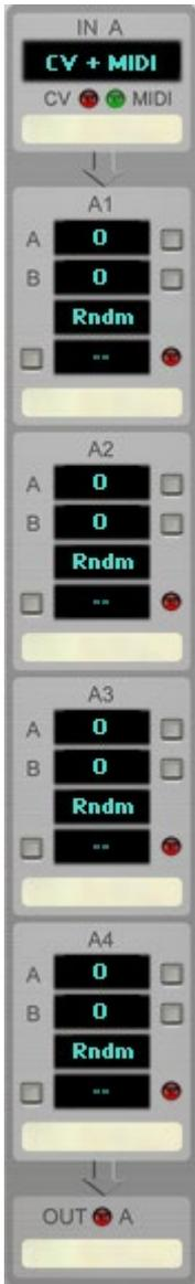
The device is divided into 8 similar columns (A to H), with an Input Selector with CV and MIDI LEDs, 4 groups of Settings (1 - 4) and a Patch Out LED indicator. With labels to help you keeping things ordered.
