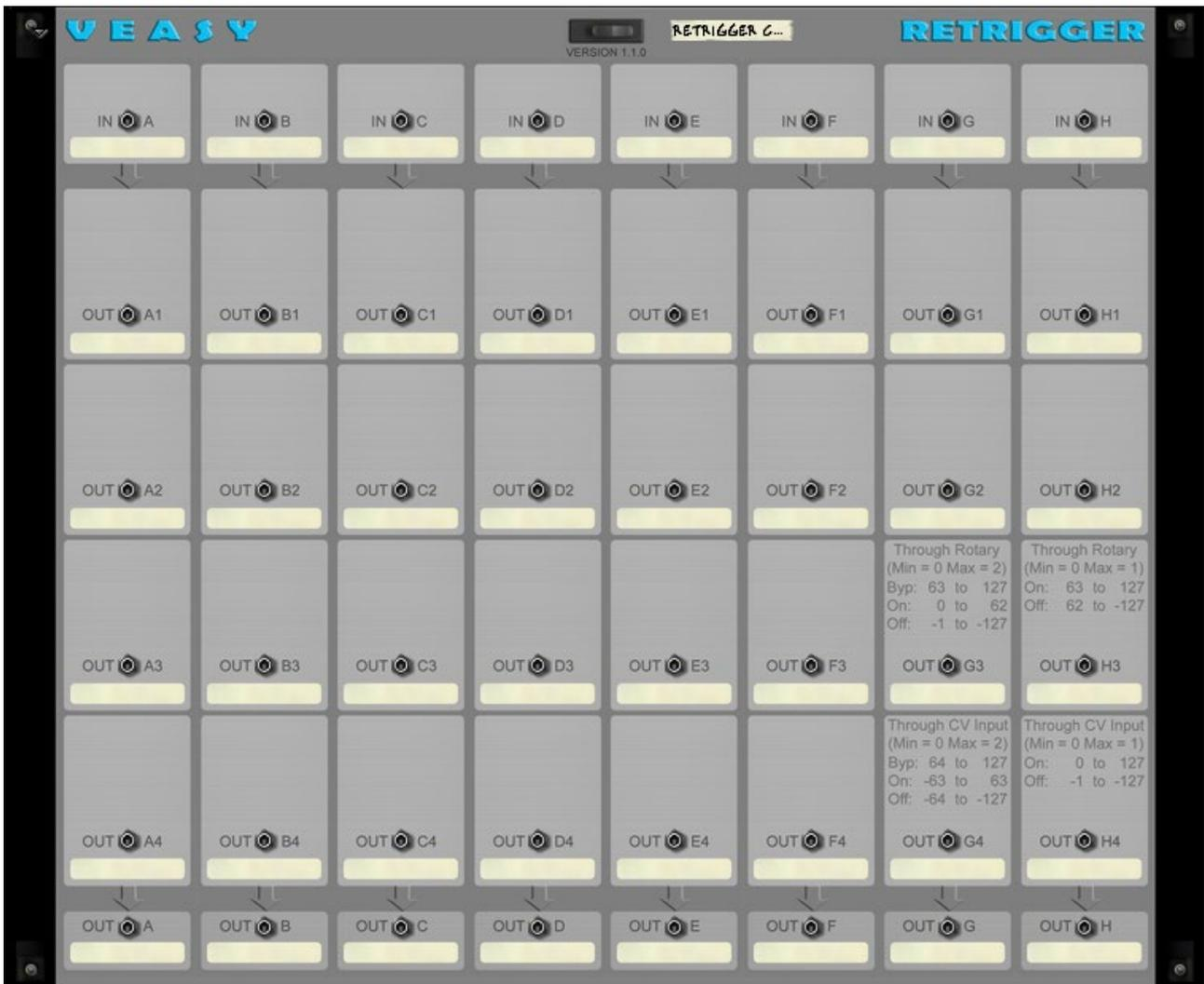
All CV Input and Output jacks are located exactly behind the corresponding Front Panel displays. So when you hold the cursor on a display you want to connect and you hit 'TAB' to flip the rack, your cursor is directly located in the right spot.
