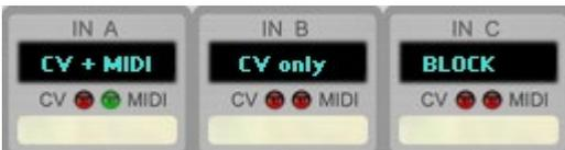
When a CV cable is connected to the CV input jack on the Back Panel, the dimmed red CV LED turns dimmed green and will light up green when input is detected. When 'MIDI Only' or 'BLOCK' is selected at the Input Selector, CV LED will turn red whether a cable is connected or not. The MIDI LED will light up green when MIDI input is detected. When 'CV Only' or 'BLOCK' is selected at the Input Selector the MIDI LED will turn dimmed red to indicate no MIDI input will be handled.
