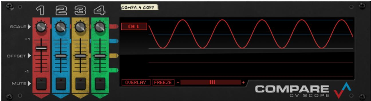
In the above image, our original sine curve has been scaled down by 50% and offset by + 0.5 V.
