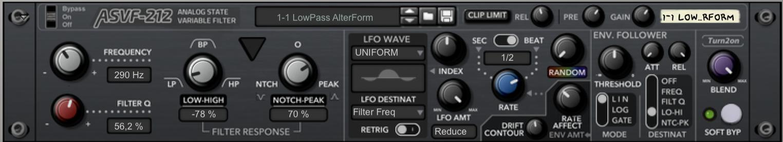
A State-Variable Filter is an active filter that uses multiple feedback techniques to produce filter responses (LowPass, BandPass and HighPass) from a single filter with user selection.
