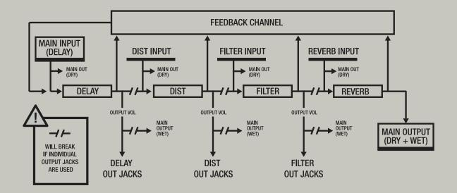
**OUROBOROS** has one stereo MAIN INPUT and one stereo MAIN OUTPUT. By default the signal first arrives in the DELAY module, once it's been delayed it moves on to the DIST, then the FILTER and lastely the REVERB before it reaches the output.
