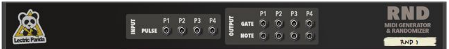
Back Panel - CV Connections
