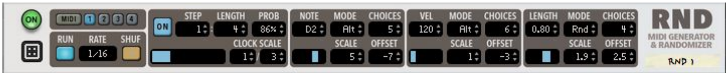
Pulse Note Generator Section Front Panel
