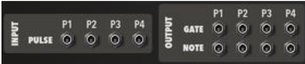
CV Connections for Pulse Note Generators
