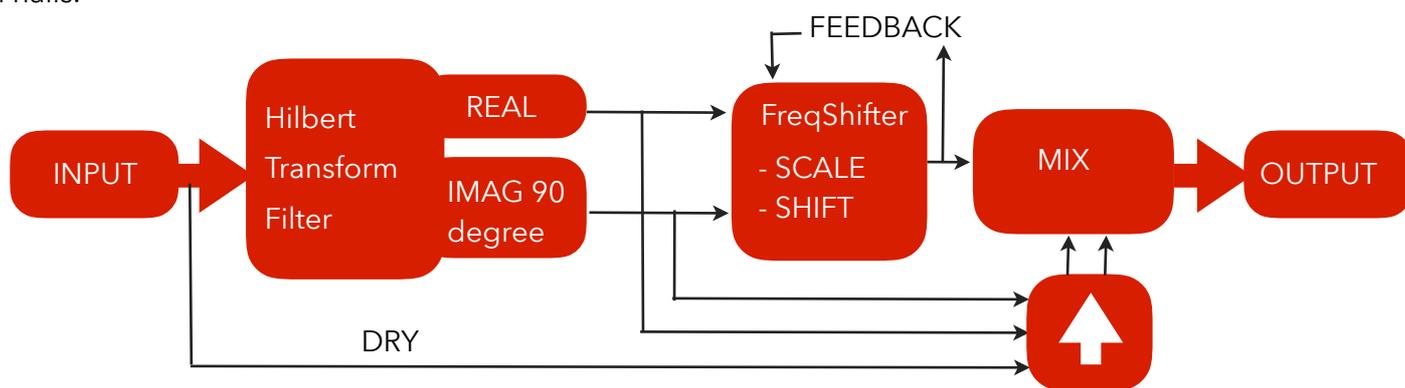
The effect uses a Hilbert Transform, that contains 2 separate channels - Real and Imaginary. Real and Imag are summed after the Frequency Shifter block where they are mixed with the dry signal.
