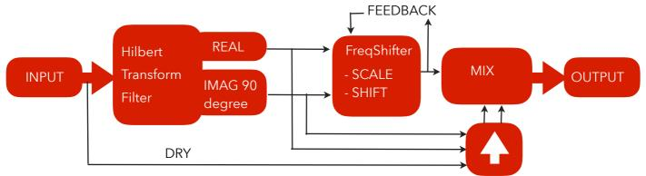
The effect uses a Hilbert Transform, that contains 2 seperate channels - Real and Imaginary. Real and Imag are summed after the Frequency Shifter block where they are mixed with the dry signal.
