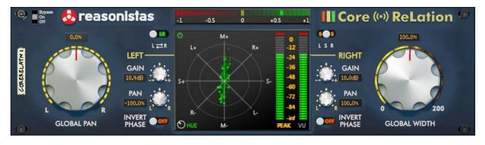
A well correlated stereo mix will be an ovular shape (tall and narrow) and centered on the vertical M axis. Here we've achieved a good overall balance between channels. Of course, the shape will vary in width and height at various points in the mix, but keep in mind the wider and shorter the shape centered on the horizontal S axis, the more phase issues you'll encounter when the mix in summed to mono.
