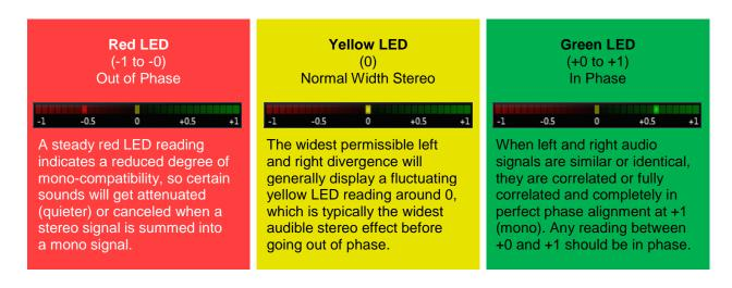
Note: We recommend using the Phase Correlation Meter in conjunction with the Goniometer for a reliable indication of mono compatibility.
