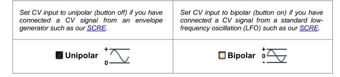
Unipolar (button off) is the default setting when a new CORE is created.
