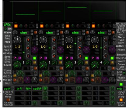
It is connecting the first 4 CV inputs to the 4 LFOs (A1 to LFO 1, A2 to LFO 2, etc.).
