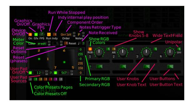
In the top middle there are four **user knobs** (with four more available via the **alt** toggle) and four **user buttons** with labels, giving you more combinator control and internal modding ability. There are also two **user pads** on the left that can be used to control various combos of the user knobs.
