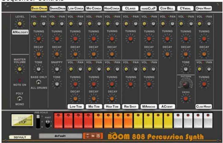
BOOM has a 16-pattern sequencer with up to 32 steps per pattern. Patterns can be automatically switched by using the automation lane on it's track. Unlike the original TR-808, BOOM is modded with a swing control, useful for everything from House to retro beats like New Jack Swing.
