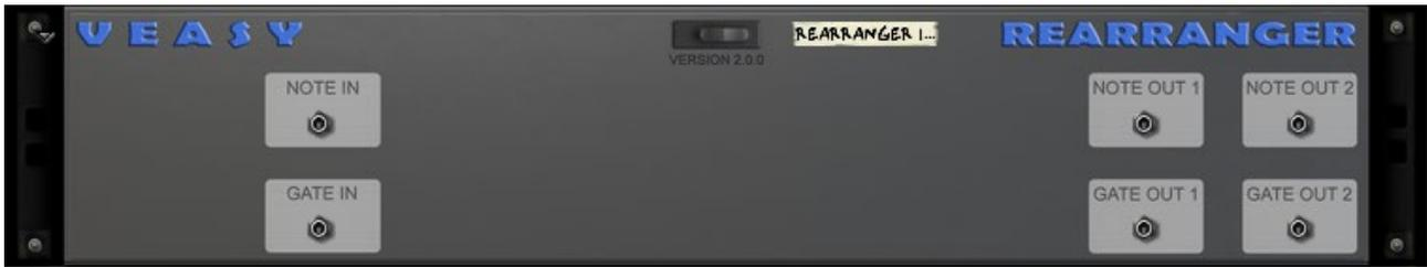
All CV input and output jacks are located exactly behind the corresponding Front Panel displays. So when you hold the cursor on a display you want to connect and you hit 'TAB' to flip the rack, your cursor is directly located in the right spot.
