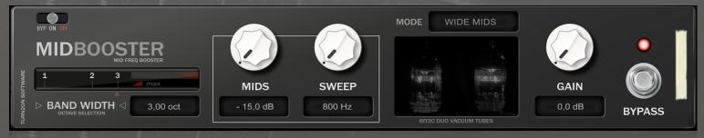
**MIDBOOSTER** is a modern parametric booster which allows adjuststments to be made to the midrange frequencies of an incoming signal using parametric tuning. It can be used in your mix to add new midrange frequencies or to cut out those which aren't required.
