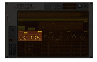
The phaser is a classic effect that uses all-pass filters (that let through all frequencies but introduces a short delay that varies with frequency) to create a sweeping/swooshing effect. Adding a small amount of phasing often adds interest to "noisy" timbres. Use the *on/off* (ON) toggle button in the upper right corner to enable the phaser.
