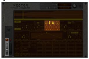
The pitch section allows you to change the tuning of the particles. The *octave* (OCT), *semitones* (SEMI), and *cents* (CENT) knobs work just like the tuning knobs in Legacy Reason synthesizers.
