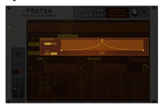
Proton has two *modulation envelopes* that allow you to construct your own LFO waveforms. To select which envelope to edit, use the ENV1 and ENV2 radio buttons.
