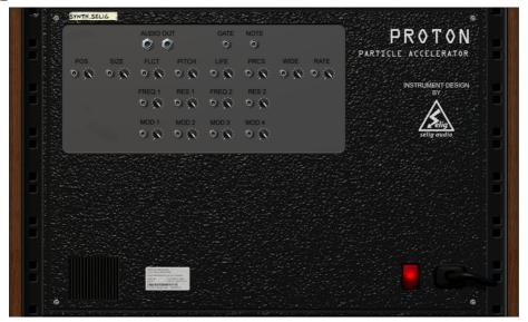
Proton's back panel has two standard L/R audio output sockets. It also has the standard Gate/Note CV inputs (which allow you to play Proton through CV utilities like Matrix or RPG-8; please refer to the Reason manual for details).
