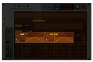
Proton has two LFOs with configurable triangle/sawtooth waveforms. When you play MIDI notes, Proton will show the current position of the LFOs by drawing a dark square (one per active voice) in the LFO displays.
