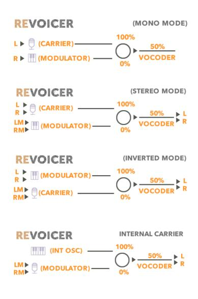
The **Classical mode** is a **Mono** Vocoder. This mode is available in **ReVoicer** when you choose Modulator source: Right Input. You can experiment with Carrier sounds with external signals by connecting your carrier signal to the Left channel. Alternatively, you can use the Internal Oscillator in ReVoicer.
