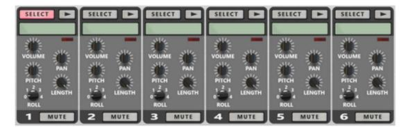
Each sample slot has a Volume, Pan, Pitch and Length setting.
