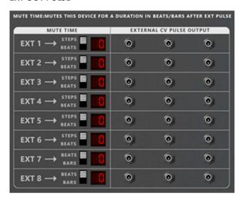
When the MOD Sequencer is set to give a pulse to one of the 8 External Outputs. All 3 outputs of that particular EXT OUT will give a pulse signal. Like the text on the back says, the mute time mutes the device for a duration after the pulse is given. This can be very useful to control other things i.e. breaks or one shots.
