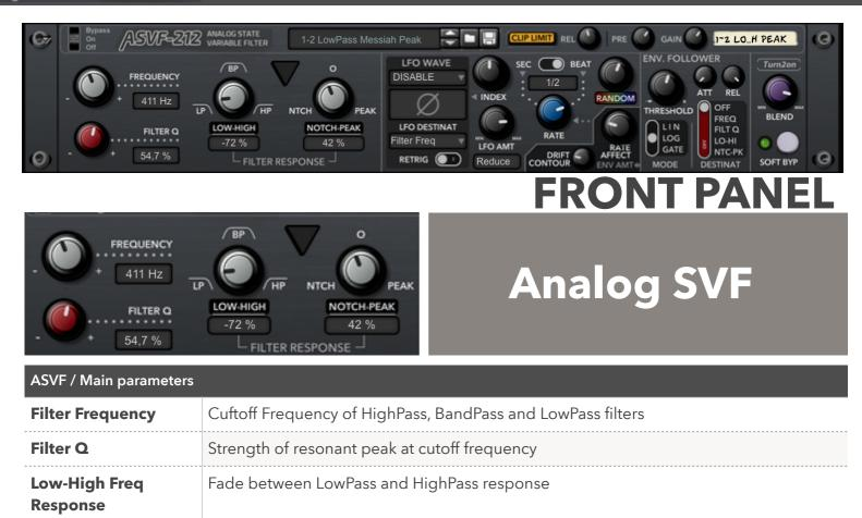
Fade between Notch/BandStop and Peak/BandPass response
