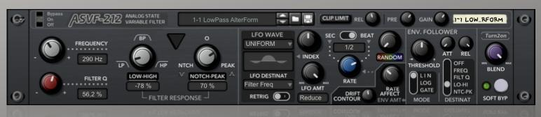
A State-Variable Filter is an active filter that uses multiple feedback techniques to produce filter responses (LowPass, BandPass and HighPass) from a single filter with user selection.
