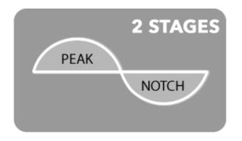
**STAGE** number determines the number of notches and peaks in 360° phase-shifting. Peak or Notch have 180° shifting.
