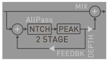
The output can be fed back to the input for a more intense effect, creating resonance by emphasizing frequencies between notches. This involves feeding the output of the all-pass filter chain back to the input. At high settings, the effect will become highly resonant, similar to a WahWah effect. **FEEDBACK** can be **inverted**, creating another variant of the effect.
