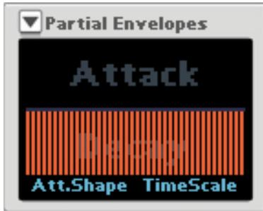
The Partial Envelopes modifier is an Attack-Decay envelope that can control the amplitude envelope of each partial in the signal individually. The Partial Envelopes display is divided into two areas: the upper area of the display where you draw the Attack times for the partials and the lower area where you draw the Decay times.
