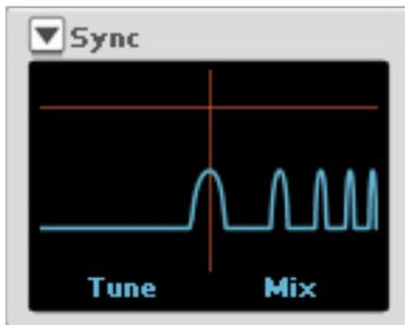
This simulates the frequency spectra of a "synced" oscillator, i.e. an oscillator (slave) that is constantly restarted at the rate of another oscillator (master). The Sync modifier creates this effect by multiplying the partials of the original signal with a factor and then interpolating and generating new harmonic partials above the original partials.
