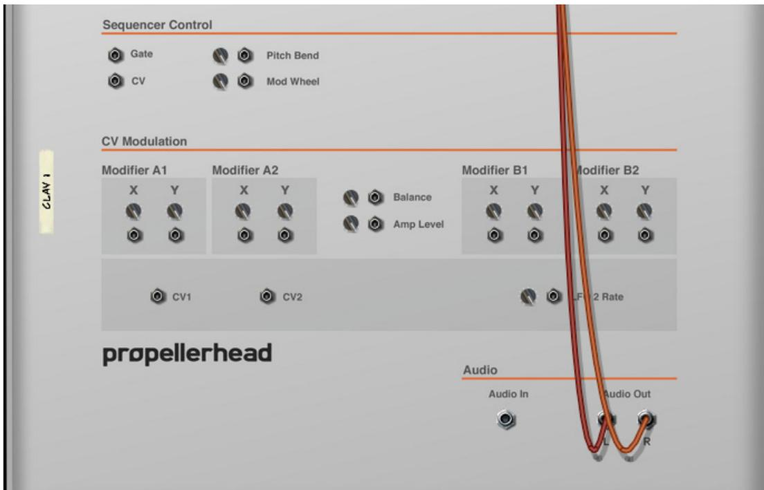
! Remember that CV connections are NOT stored in the Parsec 2 patches! If you want to store CV connections between devices, put them in a Combinator device and save the Combi patch.
