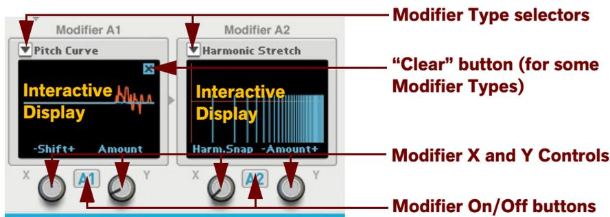
The two Modifiers in each Sound Engine control how the frequency content of the selected waveform/signal (see “Waveform/signal selector”) should be modified/affected. The modifiers are routed in series: Modifier 1 to Modifier 2.
