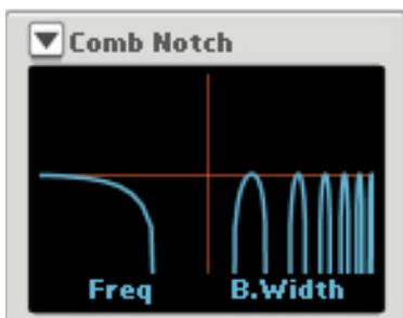
This simulates a multi notch filter, great for phaser types of effects. The filter works individually on each voice and affects the frequency content in the sound.
