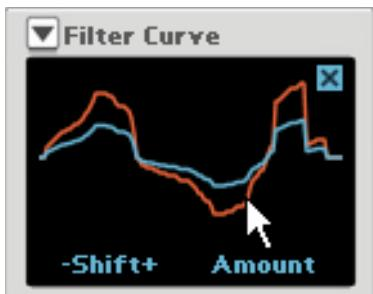
With this modifier you can design your own custom filter, by drawing your desired filter curve in the display. You can then use the X and Y knobs to change the "cutoff" frequency and the resonance/attenuation amount.
