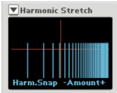
This modifier stretches or squeezes all partials (overtones) - except for the fundamental - in the signal, up or down in the frequency range.
