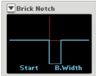
This simulates a brick wall notch filter, i.e. a notch filter with completely vertical slopes. Only the partials outside the notch pass through. The filter works individually on each voice and affects the partials in each voice.
