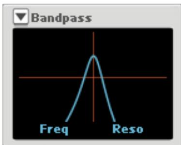
This simulates a standard 12dB/octave bandpass filter. The filter works individually on each voice and affects the frequency content in the sound.
