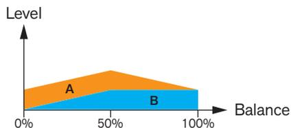
*Between 0% and 50% Sound Engine A's level is constant and between 50% and 100% Sound Engine B's level is constant.*
