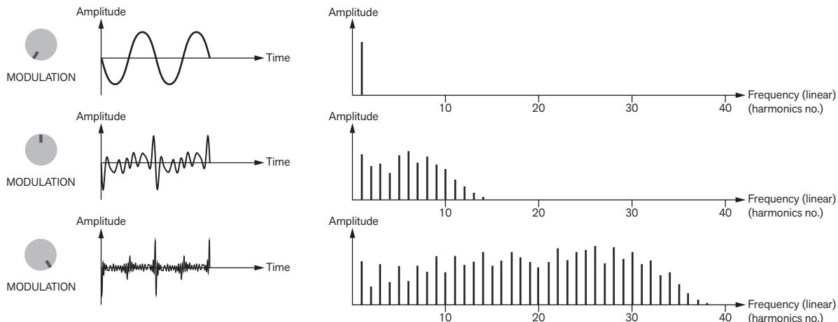
Examples of wave shapes and spectra of the FM signal when Modulation=0% (top), 50% (middle) and 100% (bottom).
