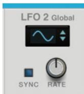
LFO 2 Global is monophonic and affects all voices together. Use the Modulation Bus to set modulation destination(s) for LFO 2, see "[The Modulation Bus section](#)".
