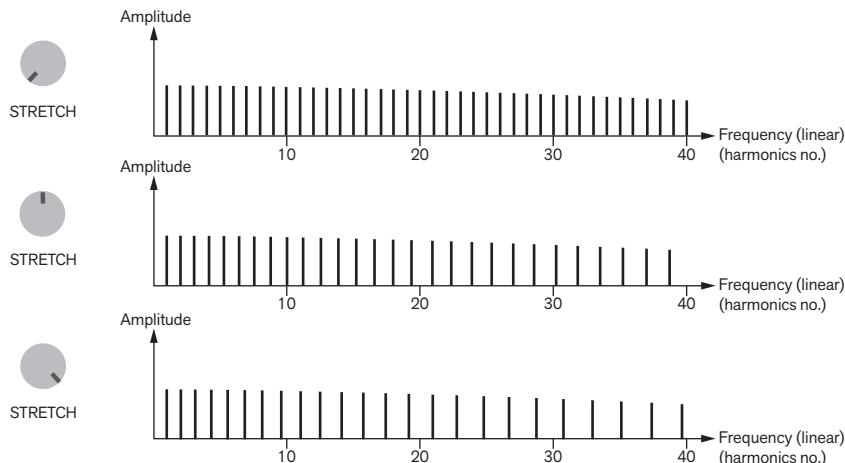
The spectra of the String signal when Stretch=0% (top), 50% (middle) and 100% (bottom).
