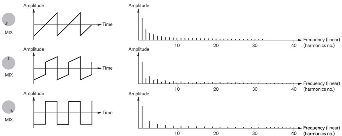
Examples of wave shapes and spectra of the Saw to Square signal when Mix=0% (top), 50% (middle) and 100% (bottom).
