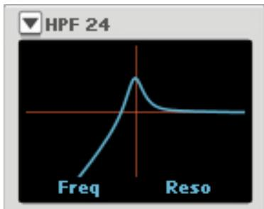
This simulates a standard 24dB/octave highpass filter. The filter works individually on each voice and affects the frequency content in the sound.
