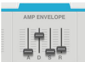
This is a standard ADSR envelope which controls the amplitude of both Sound Engines equally. The picture below shows the various stages of the ADSR envelope:
