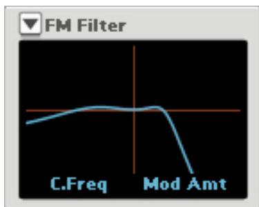
The FM Filter modifier creates a “virtual filter” which has the spectral characteristics of a frequency modulated signal.
