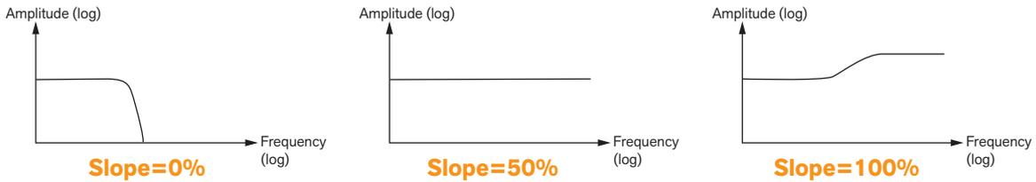
The filter attenuation/gain curves at three different Slope settings (with the same Freq setting)
