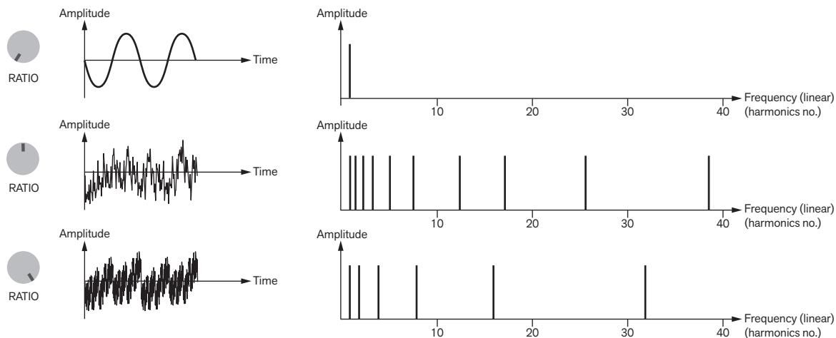
Examples of wave shapes and spectra of the Ratio signal when Ratio=0% (top), 50% (middle) and 100% (bottom).
