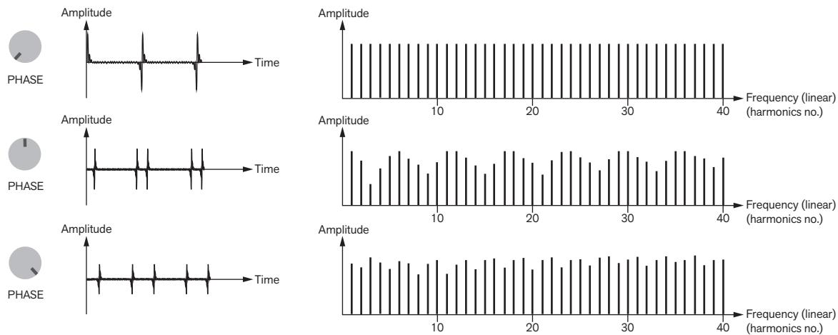
Examples of wave shapes and spectra of the Pulse signal when Phase=0% (top), 50% (middle) and 100% (bottom).
