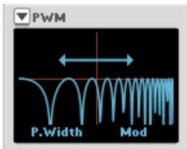
This simulates the frequency spectra you get from traditional pulse width modulation, i.e. when the pulse width of a square wave is constantly changed. Depending on what type of signal you have selected with the “[Waveform/signal selector](#)”, the character of the sound will be different. If you use a sawtooth signal the effect is almost the same as with traditional (square wave) pulse width modulation.
