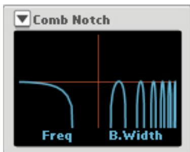
This simulates a multi notch filter, great for phaser types of effects. The filter works individually on each voice and affects the frequency content in the sound.
