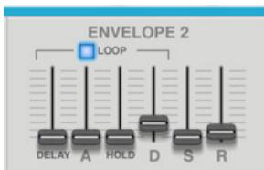
This is a polyphonic (one per voice) general purpose AHDSR (Attack, Hold, Decay, Sustain, Release) envelope with a pre-delay stage before the Attack phase. The Delay to Decay phase can also be looped. Besides the standard ADSR envelope parameters, Envelope 2 has the following additional parameters:
