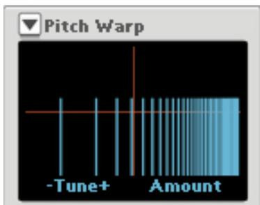
This modifier creates a copy of the signal - which can be detuned smoothly in eight steps - and tunes the pitch of the original and the copied signal, up or down, by smoothly pitch shifting all partials in the original and copied signal.
