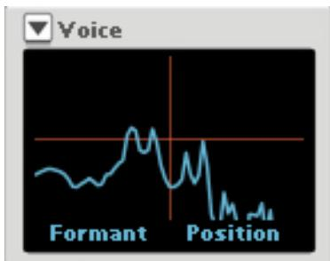
This modifier detects formants in a pre-recorded vocal sample in Parsec 2 and applies the formants to the Generator signal.
