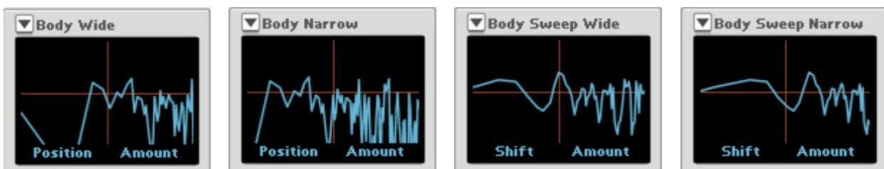
The four Body algorithms are formant filters that simulate body resonances (multi-peak+notch filters). The filters work individually on each voice and affects the frequency content in the sound.
