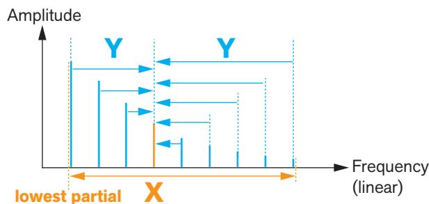
Here, the X parameter is set to the fourth partial and the Y parameter is set to 100%.
