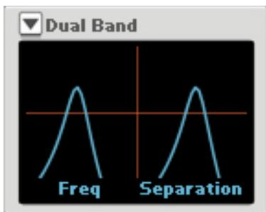
This simulates two 12dB/octave bandpass filter routed in parallel. The filter works individually on each voice and affects the frequency content in the sound.
