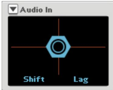
This lets you modify the Generator signal by modulating it from the Audio Input on the rear panel of Parsec 2; in practice a vocoder effect. The Audio Input signal is analyzed in real-time and the formants are applied to the Generator signal. The formants can also be shifted up and down in frequency before being applied to the Generator signal.
