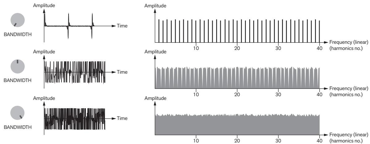
Examples of wave shapes and spectra of the Noise signal when Bandwidth=0% (top), 50% (middle) and 100% (bottom).
