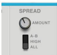
The Spread control works a little differently depending on selected waveform(s) in the Sound Engines' Generators. However, the effect is that the partials in each voice of the sound are spread in the stereo panorama in a couple of different ways.
