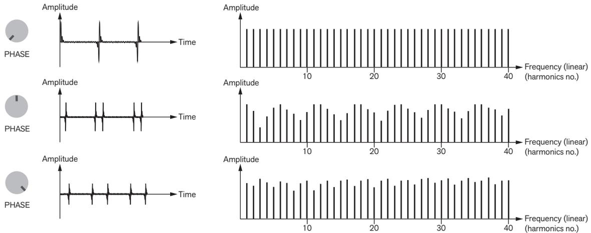
Examples of wave shapes and spectra of the Pulse signal when Phase=0% (top), 50% (middle) and 100% (bottom).
