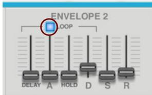
If Loop is activated, the envelope stages will loop continuously, from the Delay stage to the Decay stage, for as long as the key is held down.
