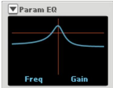
This simulates a single band parametric EQ with a fixed bandwidth. The EQ works individually on each voice and affects the frequency content in the sound.
