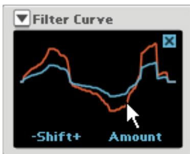
With this modifier you can design your own custom filter, by drawing in your desired filter curve in the display. You can then use the X and Y knobs to change the “cutoff” frequency and the resonance/attenuation amount.
