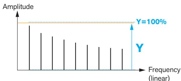
One of the Partial Filter variations (orange line) with the Y parameter at 0%, 50% and 100% (top to bottom). The grey lines represent attenuated partials or attenuated parts of partials.
