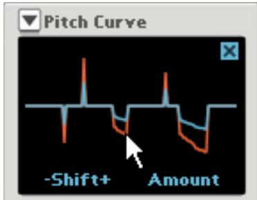
With this modifier you can pitch shift individual overtones or ranges of overtones in the signal, by drawing in your desired pitch-shift amount curve in the display. You can then use the X knob to sweep the pitch-shift curve throughout the frequency range and the Y knob to set the pitch-shift amount (deviation) of the frequencies/frequency ranges.
