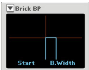
This simulates a brick wall bandpass filter, i.e. a bandpass filter with completely vertical slopes. Only the partials in the passband "window" pass through. The filter works individually on each voice and affects the partials in each voice.
