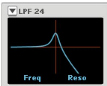
This simulates a standard 24dB/octave lowpass filter. The filter works individually on each voice and affects the frequency content in the sound.
