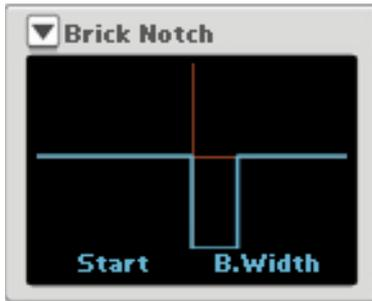
This simulates a brick wall notch filter, i.e. a notch filter with completely vertical slopes. Only the partials outside the notch pass through. The filter works individually on each voice and affects the partials in each voice.
