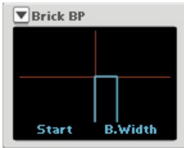
This simulates a brick wall bandpass filter, i.e. a bandpass filter with completely vertical slopes. Only the partials in the passband “window” pass through. The filter works individually on each voice and affects the partials in each voice.
