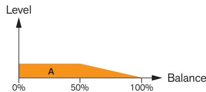
Balance levels when Sound Engine B is switched off.
