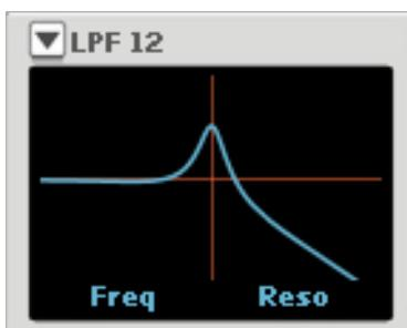
This simulates a standard 12dB/octave lowpass filter. The filter works individually on each voice and affects the frequency content in the sound.
