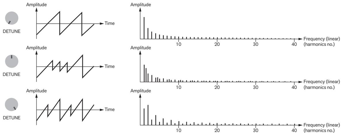
Examples of wave shapes and spectra of the Dual Saw signal when Detune=0% (top), 50% (middle) and 100% (bottom).
