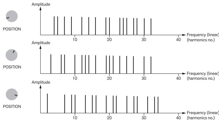
The spectra of the Sparse signal at three different Generator knob (Position) settings.
