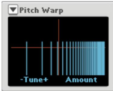
This modifier creates a copy of the signal - which can be detuned smoothly in eight steps - and tunes the pitch of the original and the copied signal, up or down, by smoothly pitch shifting all partials in the original and copied signal.
