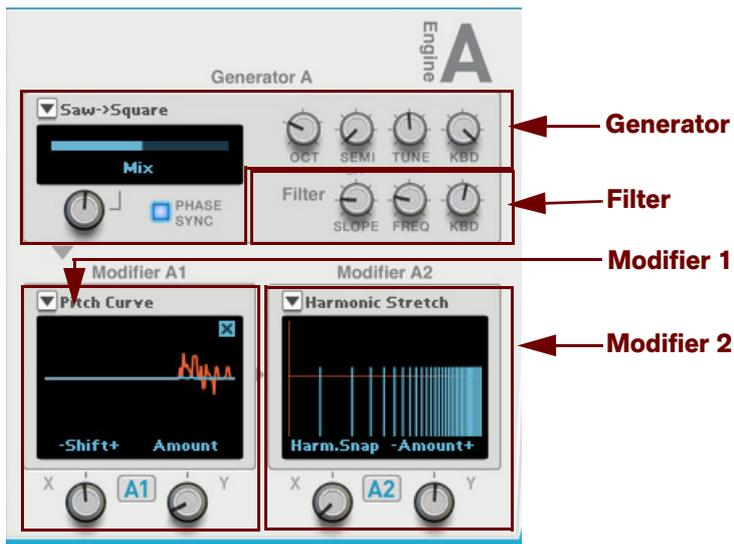
Parsec 2 features two Sound Engines. These could be considered very advanced and flexible sine wave generators. Each Sound Engine can generate up to 512 sine wave signals. The sine wave signals of each Generator can be modified via two Modifier sections, Mod 1 and Mod 2, and their dynamic X and Y controls.
