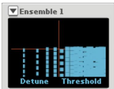
This is the perfect modifier for really dense pad sounds! The Ensemble 1 modifier simulates a type of chorus effect by utilizing noise modulation of the partials. The Ensemble 1 modifier is best suited for sounds with slow attacks, since the noise modulation always starts from zero and the transients are therefore "smeared out". The modifier works individually on each voice and affects the partials in each voice.
