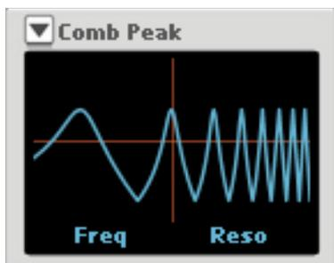
This simulates a comb filter with a positive feedback loop - but without feed forward - ideal for flanger and phaser types of effects. The filter works individually on each voice and affects the frequency content in the sound.
