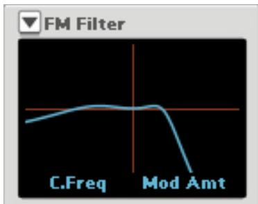
The FM Filter modifier creates a "virtual filter" which has the spectral characteristics of a frequency modulated signal.
