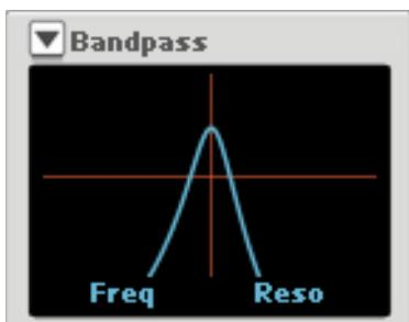
This simulates a standard 12dB/octave bandpass filter. The filter works individually on each voice and affects the frequency content in the sound.
