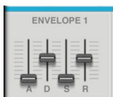
This is a polyphonic (one per voice) general purpose ADSR envelope generator (see the description above) which can be assigned to control selectable parameter(s) in the Modulation Bus section. For example, you can assign it to control the X and Y parameters in the desired Sound Engine Modifier algorithms.
