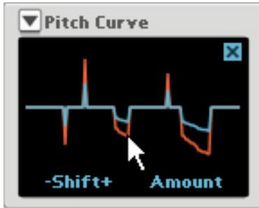
With this modifier you can pitch shift individual overtones or ranges of overtones in the signal, by drawing in your desired pitch-shift amount curve in the display. You can then use the X knob to sweep the pitch-shift curve throughout the frequency range and the Y knob to set the pitch-shift amount (deviation) of the frequencies/ frequency ranges.
