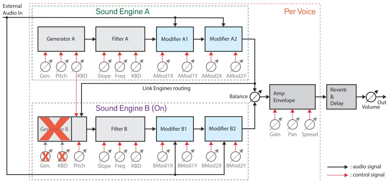
Parsec 2 signal flowchart in “Link Engines” mode.
