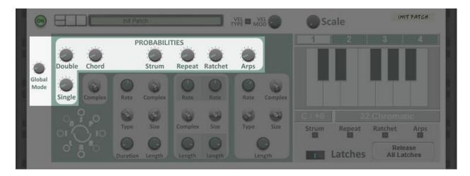
The starting point for where the decisions are made in Inspiral is the Global Mode control on the left-hand side of the device.
