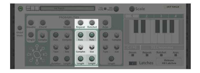
The Note Repeat and Ratchet functions are simpler than the Strums and the controls mirror those in the Strum section, only there is no need for a type or a duration control with these.
