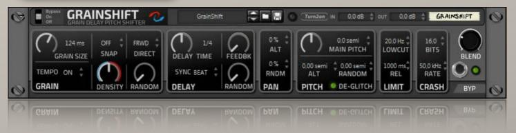
Introducing a powerful granular effect for real time processing of audio signals with pitch-shifter and delay. With **GRAINSHIFT** you can select the position and length of grains that you get from the incoming signal, as well as the playback direction of grains that can be pitch-shifted and mixed with the dry signal.
